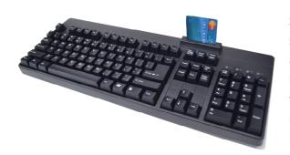
The Digimore Heavy-duty Smart Card USB Keyboard, KB-6868-SCR is design for use with smartcard enabled identification system. It is ideal for providing user authentication for applications such as network login, e-government, e-commerce, healthcare and etc. This keyboard works with all smart cards that comply with ISO 7816 Class A, AB and C memory and microprocessor smart cards (T=0, T=1). Antimicrobial ABS material (option) is also available upon requested.
