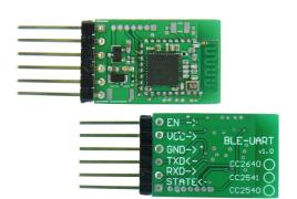
The *DM-U08* is Central and Peripherals 2-in-one Bluetooth UART Serial pass-through module. Users can change roles (Central and Peripheral mode) and serial baud rate and device name via AT command. Parameters such as name and password are flexible to use.
