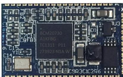
The **ABT01B** is a Bluetooth HID module using Broadcom Bluetooth 3.0 controller **BCM20730**. This module is ideal for wireless sensing device applications including pointing devices like mice, trackball, gestural controls or keyboards, leisure equipment, consumer electronics, HID, health care, etc.. The module is integrated with EEPROM, PCB antenna and crystal to reduce the external BOM cost.
